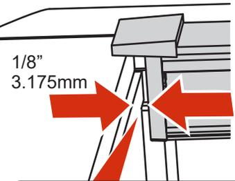
Rails are designed to be spaced 1/8" from factory tailgate/tailgate cap. Some trimming or modification of plastic drop-in liners or BedRug style products may be required.
