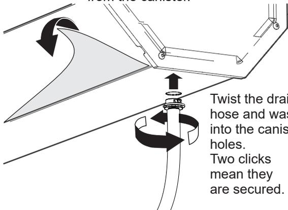
Twist the drain hose and washer into the canister holes. Two clicks mean they are secured.
