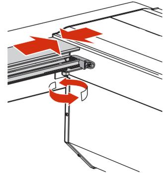
**4** Slide the assembled cover and rails back toward the tailgate. The rail ends should be 1/8", 3.175mm from the tailgate.
