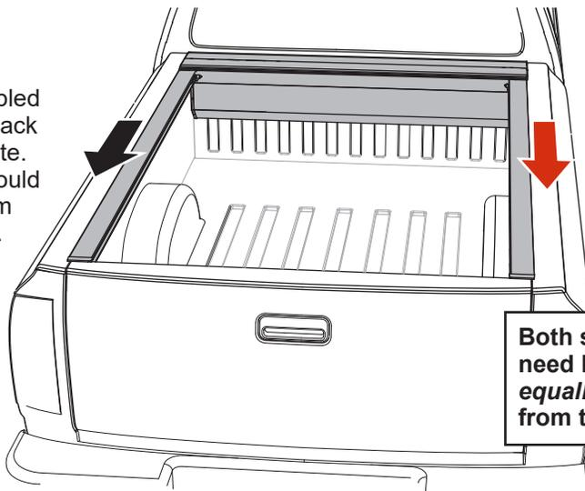
Both sides need be *equally* spaced from the tailgate.
