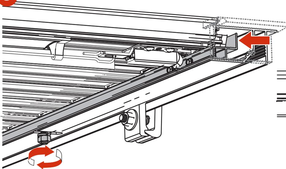
The rail end cap is shown as transparent to better show the inner rail. Use the mounting bolt to push the inner rail inward to contact the cover. Tighten all of the mounting bolts to 6.7 ft-lbf, 9,1 N-m. Align and tighten both sides.
