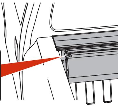
**2** Make sure that the front/cab end seal is pulled forward and seals along the bulkhead.
