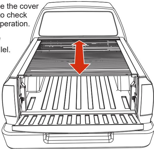
**9** With the cover mounted and parallel the rear seal needs to be trimmed to match the rail end cap. Both sides.
