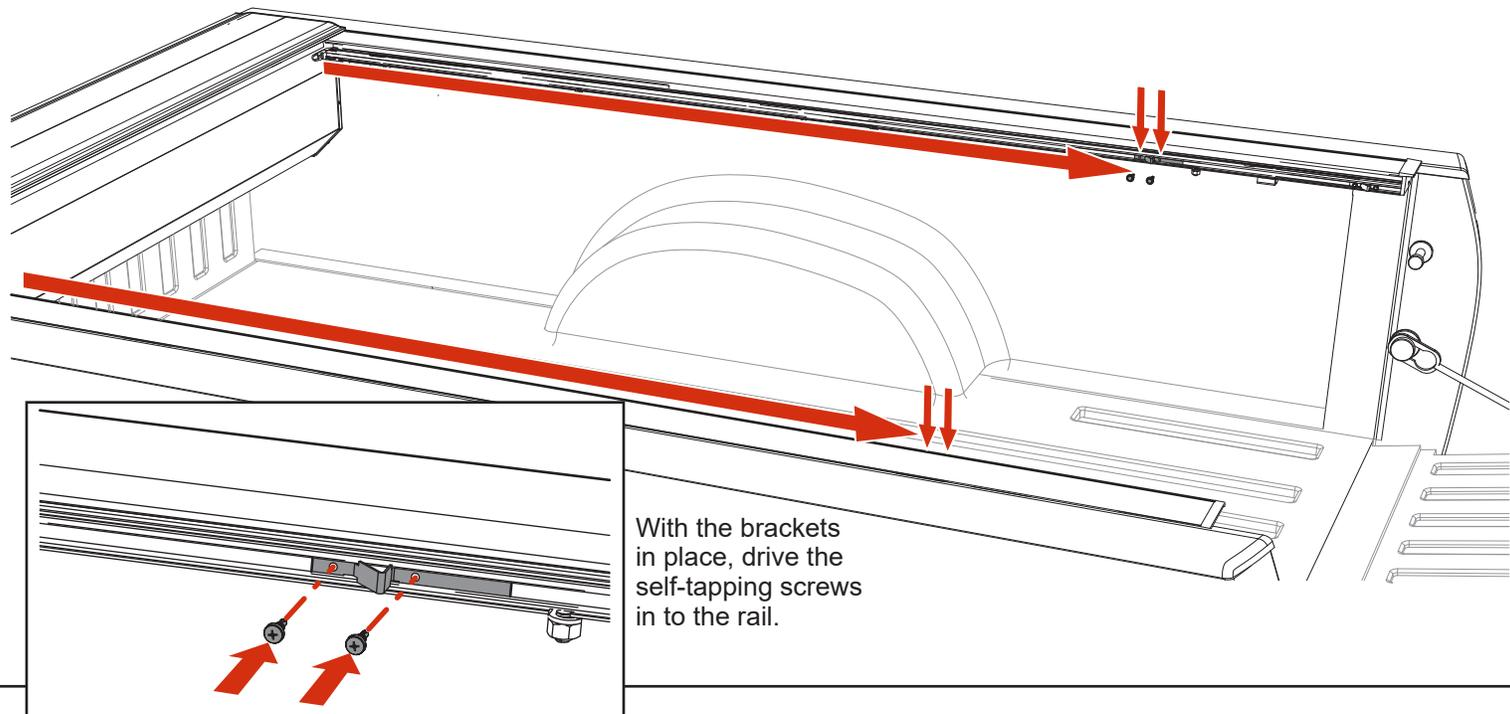
**6** Align and tighten the inner rails with the cover closed.
