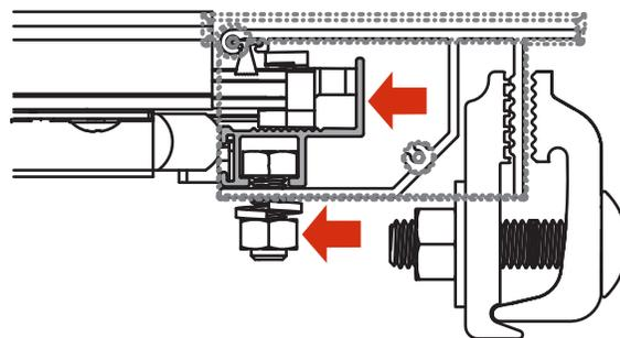
**7** Check the proper latch engagement on both sides.
