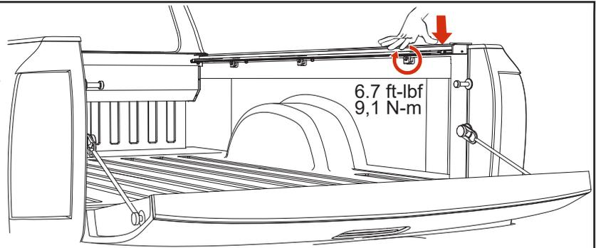
Position the front clamp 12", 305 mm from the canister. The rear clamp 12", 305 mm from the tailgate. For long beds place the center clamp centered between the front and rear clamps. Tighten the clamps, push down on the rail while tightening.
