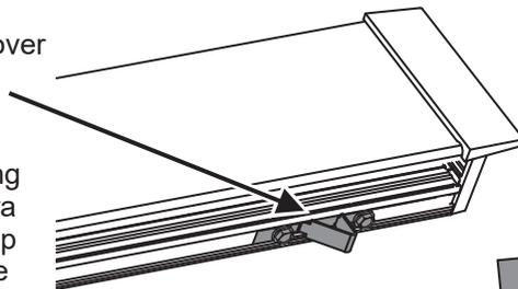
If you would like to add these additional cover stops, slide the provided stop brackets into the open end of the cover rail before installing the rails.
