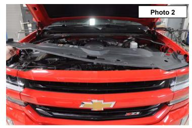
3. Remove the four bolts on top of grill. Then pull on the bottom of grill to get clips to release. Remove grill. See Photo 3 & 4.
