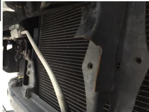
**Step 3:** Carefully push AC line back towards radiator to ensure there is no contact with RDS bumper. *Fig. C*
