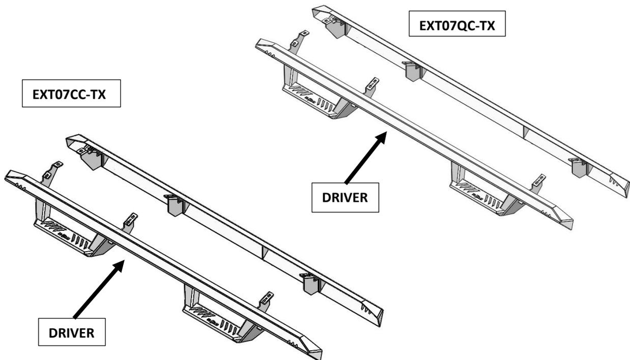
**Step 2:** Install three rocker panel brackets to the attachment points located on the backside of the channel using the supplied 3/8" x 3/4" carriage bolts and 3/8" flanged nuts. Leave finger tight for now.
