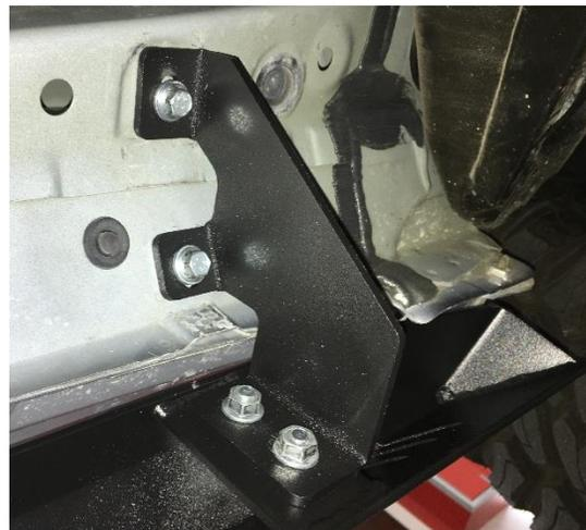
**Step 6:** Next, adjust the step assembly up/down and front/back to level out the step rail with body panel and then tighten step to brackets at 30 ft. /lbs.
