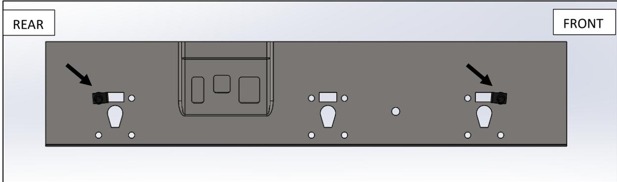
**Step 2:** Next, install (x2) of the supplied Rocker panel mounting brackets to the factory mounts using the 3/8"x1" Hex bolt, 3/8" USS Flat washer for the upper attachment and the 3/8"x 1 1/2" carriage bolt 3/8" Hex nut and 3/8" USS washer for the lower attachment. Leave loose for now. **NOTE: The carriage bolts will start from the outside of the body, the nut and washer will be only visible from underneath the vehicle.**
