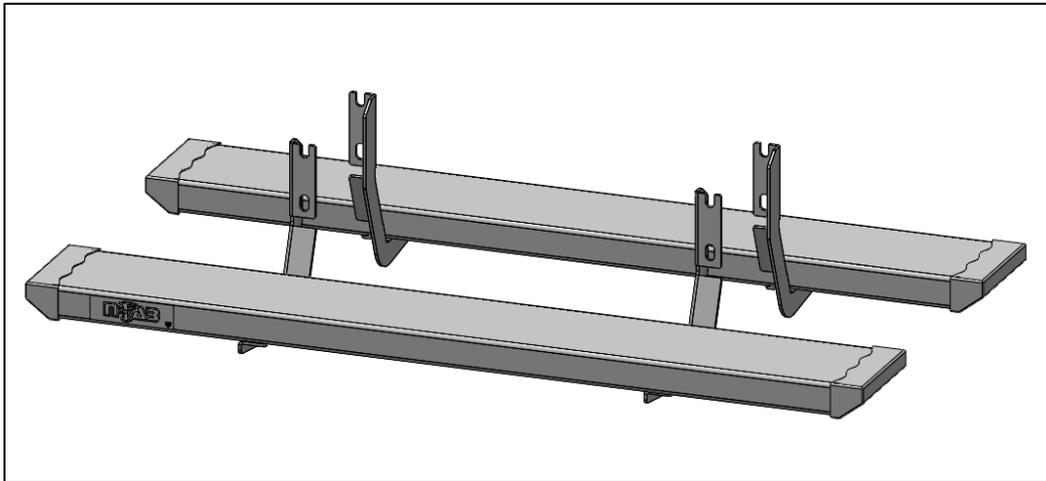
**Step 1:** Starting with the Driver side, locate the holes for the upper mounts (x2) and install the supplied (x2) 3/8" clips in each position. See below for configuration.
