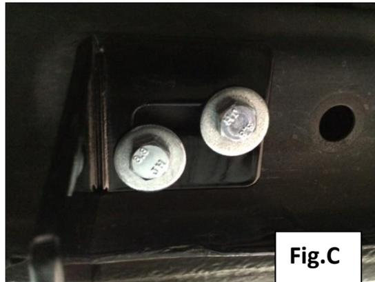
**Step 4:** Move to the front bracket and insert hardware finger tight and then to the rear bracket.
