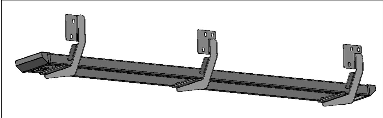
**Step 5:** Insert the supplied threaded brackets x3 inside the running board lip over the top of each bracket.
