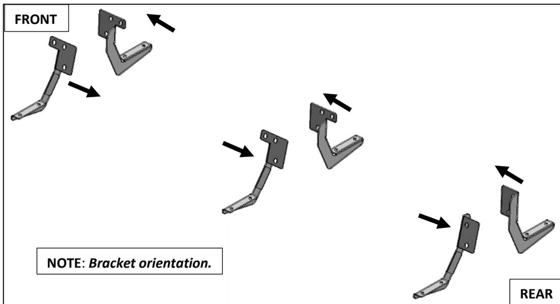
**Step 4:** Set running board along the top of all three brackets and center along the cab.
