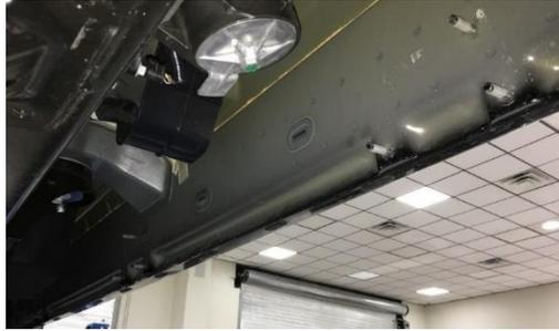
**Step 2:** On the inside rocker panel there will be three 8mm studs coming out from the panel. These studs may be covered in paint and will need to be cleaned before the installation.
