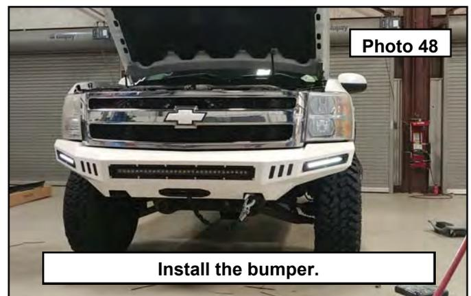
56. Install the winch fairlead using the provided 12mm button head bolts from the bumper hardware bag. Torque to 30 ft-lbs. If you are not using a winch, install the winch block off grill using the 12mm button head bolts and 1/4" thick spacers. Line up until all the gaps are even and torque the bolts to 5 ft-lbs.
