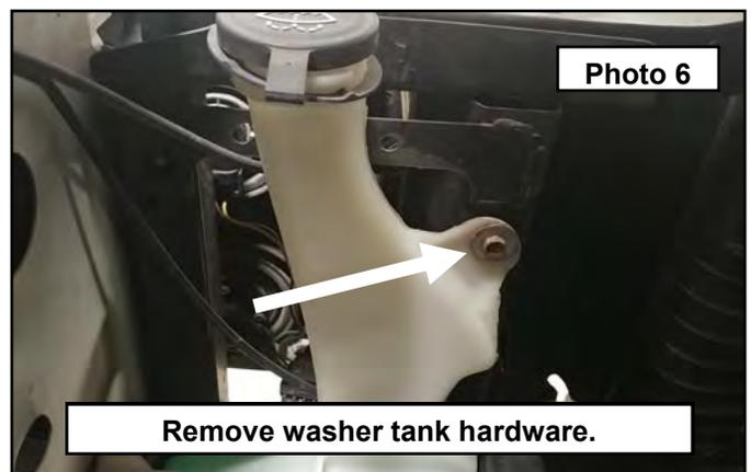
11. In the driver wheel well, remove the washer tank bolt using a 10mm socket and plastic push pin. **Photo 7**
