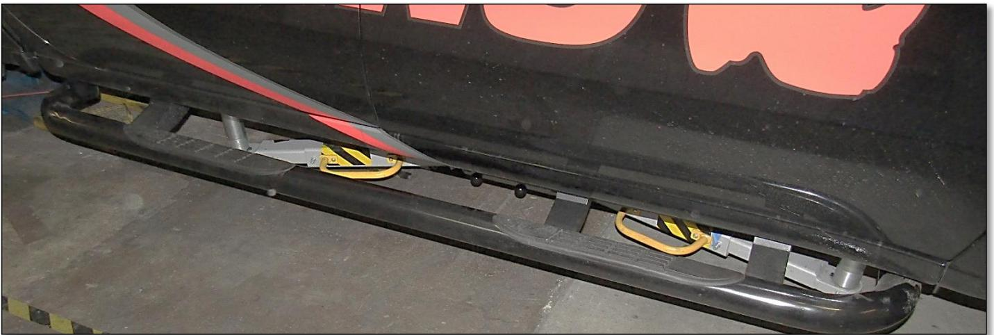
**Step-6** Repeat the installation steps to install the mounting brackets and step on the driver side.
