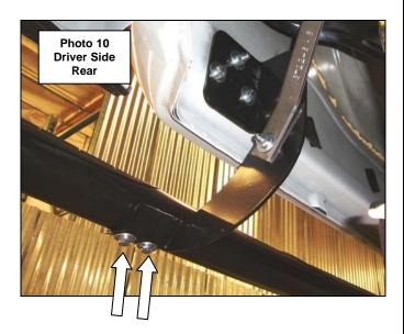
**Step-10** Align the side step with the vehicle and tighten all factory, side step and bracket nuts and bolts. Repeat the installation steps to install the passenger side brackets and side step.
