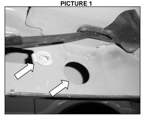
Insert into round hole a steel bar with 1/2" bolt and place in the square hole a 3/8" clip nut as shown. Front driver's side picture.
