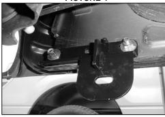
Rear mounting bracket placed. Rear driver's side shown.
