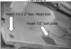
Insert into the largest round hole a 1/2" bolt plate and place into the small round hole shown a 1/2 x 2" hex head bolt
