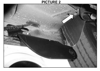
Insert into the square hole steel bar with 5/16" bolt. Front driver's side picture.
