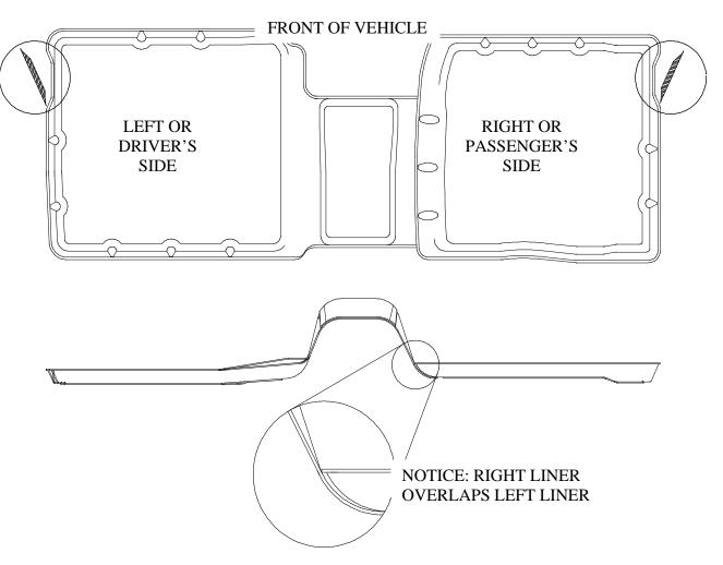
JEEP CHEROKEE OWNERS WITH THE 2-DOOR MODEL WILL NEED TO TRIM THEIR LINERS AS SHOWN CIRCLED ABOVE TO ACCOMMODATE THE FRONT SEAT BELT ATTACHMENT POINTS. A UTILITY KNIFE OR HEAVY SCISSORS WORK WELL FOR TRIMMING YOUR LINERS.
