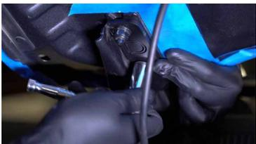
5. Secure the bracket and hood hinge by tightening the factory bolts, ensuring the hood hinge lines up with the tape.
