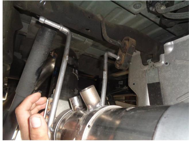
**Step 2. 2014-2020 Installation:** Begin installation of the Magnaflow system by clamping the extension pipe to the newly cut outlet of the DPF using the supplied 4.00" clamps and fitting the hangers in the rubber insulators (leave all clamps loose for final adjustment of the complete system). If your vehicle has any sensor(s) re-install at the appropriate locations. Any boss that doesn't get a sensor installed into it must be closed off with a provided screw in plug.
