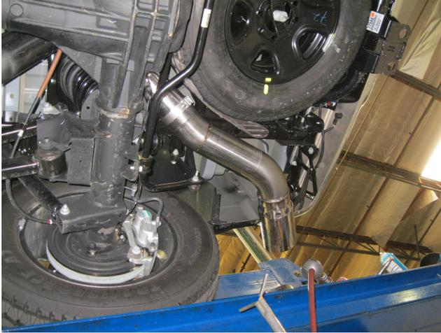
**Step 4.** Complete the installation by sliding the specified Rear Hanger Clamp Assy onto the Tailpipe Assy and attaching the Tailpipe Assy to the Over Axle Pipe. Engage the hangers into OE rubber insulators.
