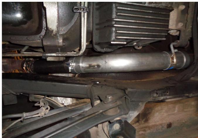
**Step 2.** Install the corresponding Inlet Pipe Assembly and loosely fasten it to the turbo charger outlet using the OEM clamp. Next, loosely attach the Inlet Pipe Lower Assembly to the Inlet Pipe Assembly using the supplied clamp. Refer to the table below to select the appropriate extension pipes for your vehicles configuration.
