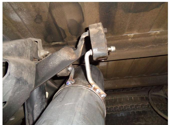
**Step 4.** Loosely install the Over Axle Pipe Assembly using the supplied clamps. Locate both hangers to the rubber insulators.
