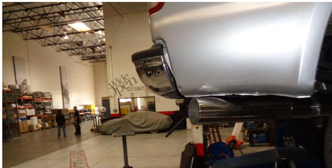
**Step 6.** Once a final position has been chosen for the new exhaust system, evenly tighten all clamps from front to rear using the torque specifications on page one of the instructions. Inspect all fasteners after 25-50 miles of operation and re-tighten if necessary.
