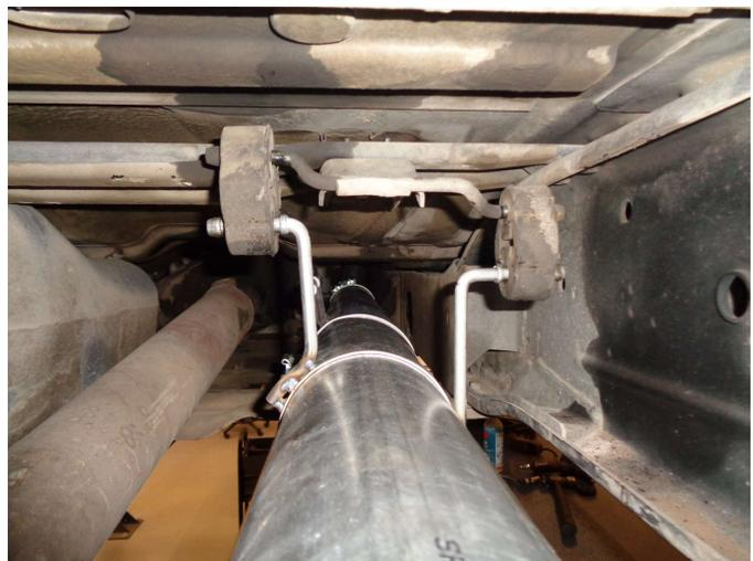
**Step 3.** As you assembly the Extension Pipes loosely locate the Hanger Clamp Assemblies as needed.
