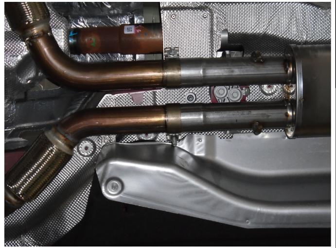
Step 3. Install the new Muffler Assembly to the Inlet Pipes using the supplied clamps. Engage the welded hangers to the rubber insulators.
