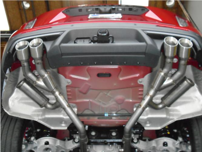
Step 5. Install the new Tail Pipe Assemblies to the Mid Pipes using the supplied clamps. Engage the welded hangers to the rubber insulators.
