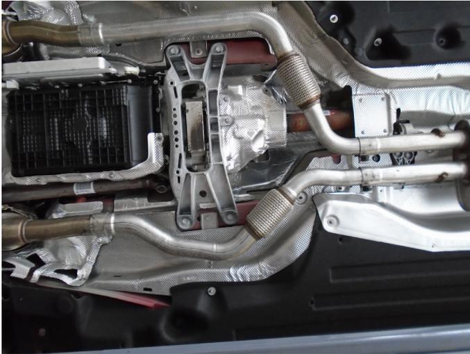
Step 1. Remove the OEM system by first loosening the clamps attaching the stock muffler to the Inlet Pipes. Next loosen the clamps attaching the Inlet Pipes to the catalytic converters. Next, Disengage all welded hangers from the rubber insulators. The exhaust system can now be removed. Retain all fasteners and insulators as they will be needed to mount your new MAGNAFLOW system.
