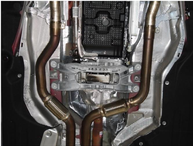
Step 2. Install your new system by first attaching the new Inlet Pipes to the catalytic converter outlets using the supplied clamps. Keep all clamps loose to allow for final adjustment.
