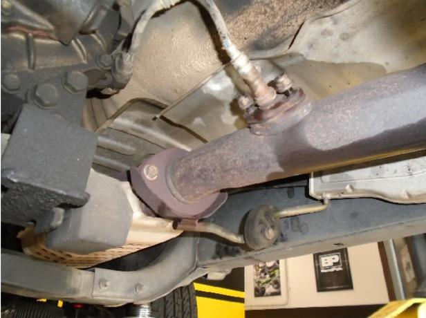
**Step 1:** To remove the OEM exhaust system, unfasten hardware at the muffer flange and remove the O2 sensor and secure out of the way (Retain both flange fasteners to be re-used).
