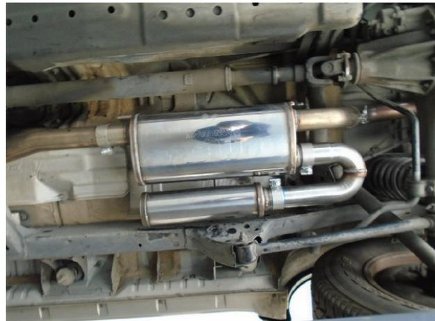
**Step 4:** Next attach the Oval Muffer to the Inlet Pipe with the supplied 2.50" clamp. This exhaust system is configured to allow the user to tune the sound. For a more moderate exhaust sound install the U-pipe Assy and the 4.00" NDT Chamber (as shown) using the supplied 2.50" clamps. For a more aggressive sound see configuration chart below.
