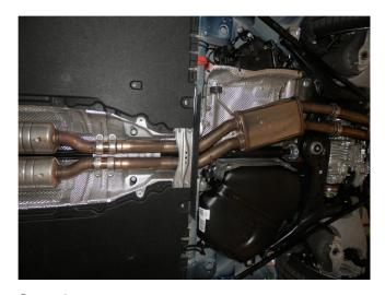
**Step 3.** Begin installation of the new system by fastening the Resonator Assembly inlets to the catalytic converters using the OEM clamps and fitting the hangers into the rubber insulators (Leave all clamps and fasteners loose for final adjustment of the complete system.)
