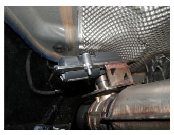
**Step 2.** Once the OEM system is on the ground you will need to swap the servo motors from the factory control valves to the control valves on the Magnaflow Tip Assemblies. Use the new supplied hardware to attach the servo motors the the valves.
