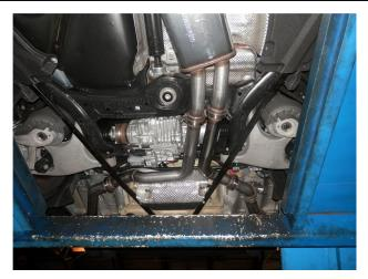
**Step 4.** Next attach the Mid Pipes to the outlets of the Resonator Assembly using the supplied V-Band clamps. \*\*NOTE: Take care when using the V-Band Clamps, they are designed for one time use only. Once the clamp is tightened it can not be reused.
