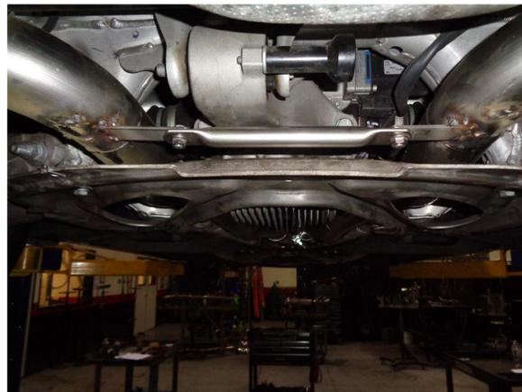
**Step 3.** Next slip the inlet of both Mid Pipes over the outlets of the Resonator Assembly and loosely secure using the supplied clamps, loosely install the brace using the OE fasteners Install the two Tail Pipe Assemblies in a similar fashion. Locate the welded hangers to the rubber insulators.
