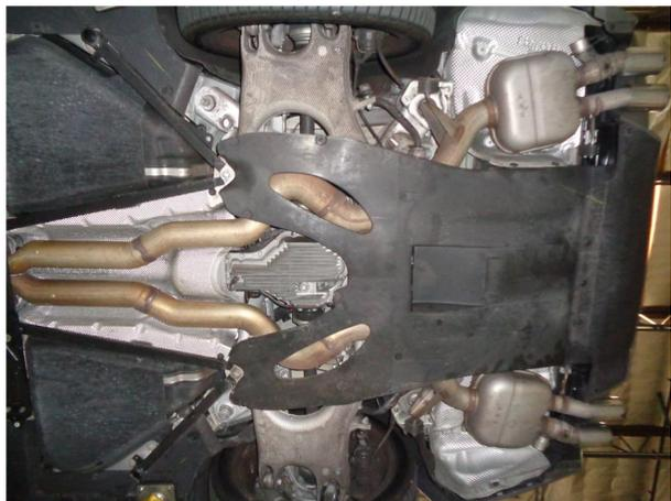
**Step 1.** To remove the OEM exhaust system begin by removing the frame cross brace, the exhaust brace and cover at the rear of the vehicle. Also unfasten the ground strap located on both muffler assemblies. Next unbolt the inlet pipe flanges at the catalytic converters. Working front to rear with the exhaust supported disengage or unfasten all hangers and remove the exhaust. Retain all hardware and insulators as they will be use to install the new system.
