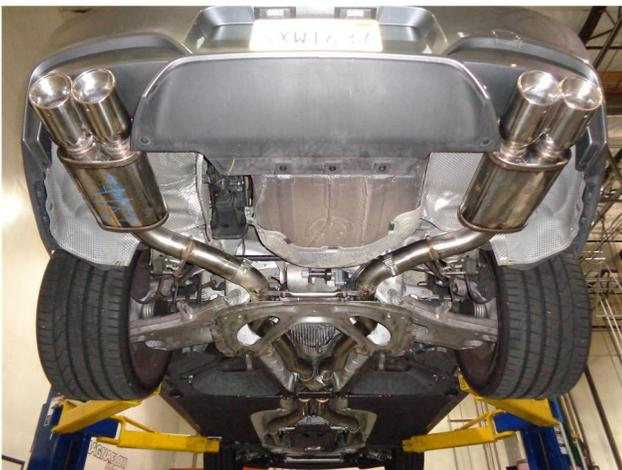
**Step 5.** Once a final position has been chosen for the new system, evenly tighten all clamps from front to rear using the torque specifications on page one of the instructions. Inspect all fasteners after 25-50 miles of operation and re-tighten if necessary.
