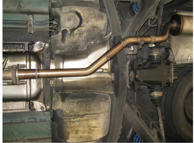
**Step 2.** Begin installation of the new system by fastening the Inlet Pipe Assembly to the catalytic converter outlet using the OEM fasteners and inserting the hanger into the rubber insulator (Leave all clamps and fasteners loose for final adjustment of the complete system).
