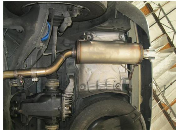
**Step 3.** Next Install the Muffler Assembly to the Inlet Pipe using the supplied 2.00" clamp. Insert hangers into rubber insulators.
