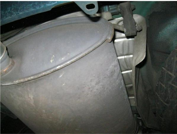
**Step 1.** To remove the OEM exhaust system begin by un-fastening the flange located behind the catalytic converter and disengaging all welded hangers from the rubber insulators. Do not damage or discard the rubber insulators or fasteners as they will be re-used to mount the new system. Working front to rear remove the exhaust from the vehicle.
