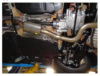
**Step 2.** Begin removal of the OEM system by loosening the slip clamp at the vehicles exhaust inlet. Working front to rear disengage all welded hangers from the rubber insulators. Be sure to retain all mounting hardware as it will be needed to mount your new MAGNAFLOW exhaust.
