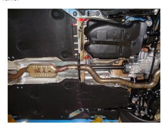
**Step 5.** Loosely attach the Inlet Pipe Assembly to the OEM slip clamp. Engage the welded hangers to the rubber insulators.
