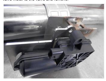
**Step 4.** Before installing your new exhaust system attach the OEM valve motors to each valve using the supplied hardware. The alignment spring on the motor will need to be engaged into the keyway slot of the new valve.
