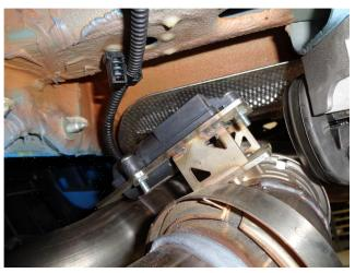
**Step 6.** Loosely install Muffler Assembly using the supplied V-Band clamp. Attach the welded hangers to the rubber insulators. Re-attach both electrical connectors to the exhaust valve motors. \*\*NOTE: Take care when using the V-Band Clamps, they are designed for one time use only. Once the clamp is tightened it can not be reused.
