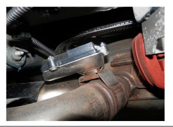
**Step 3.** Once the OEM exhaust system has been removed undo the three nuts attaching each exhaust valve motor to the valve and remove.
