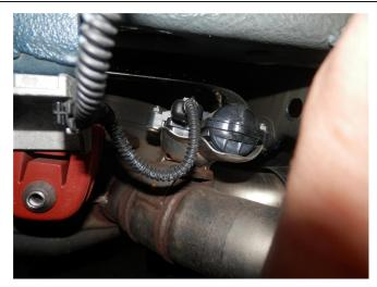
**Step 1.** Before removing the OEM exhaust system you will need to unplug the electrical connectors for both exhaust control valves. These are located on the vehicles tail pipes.
