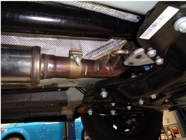
**Step 2.** Begin installation of your new MAGNAFLOW system by slipping the Resonator Assembly inlet end over the Catalytic Converter outlet locating the alignment pin into the corresponding slot on the Resonator inlet. Loosely secure using the supplied 2.25" clamp. Leave all clamps loose during initial installation.
