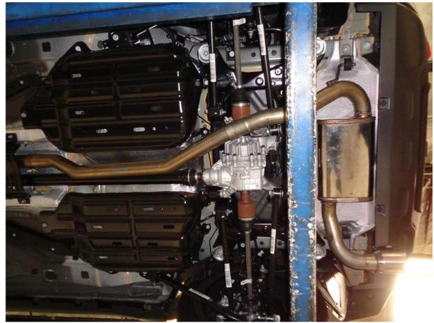
**Step 3.** Next, attach the Mid Pipe to the Resonator Assembly outlet using the supplied 2.50" clamp.
