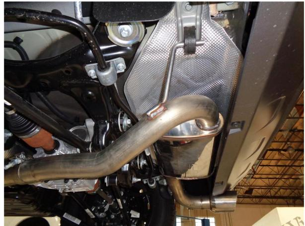
**Step 4.** Mount the Muffler Assembly to the Mid Pipe with the supplied 2.50" clamp and locate both welded hangers into the OEM rubber insulators.
