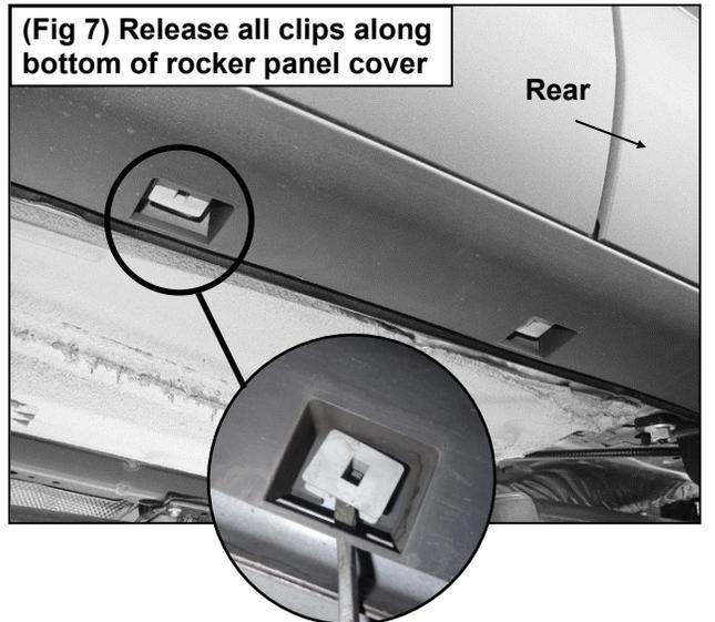
(Fig 7) Release all clips along bottom of rocker panel cover
