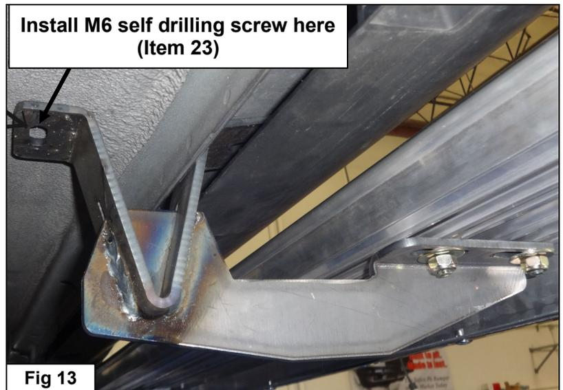
Install M6 self drilling screw here (Item 23)
