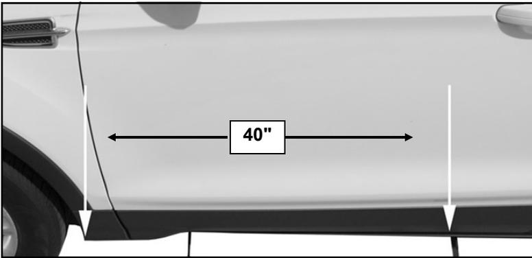
(Fig 8) Measure approximately 40 inches from bottom corner of wheel opening along rocker panel to locate factory hole for center Bracket
