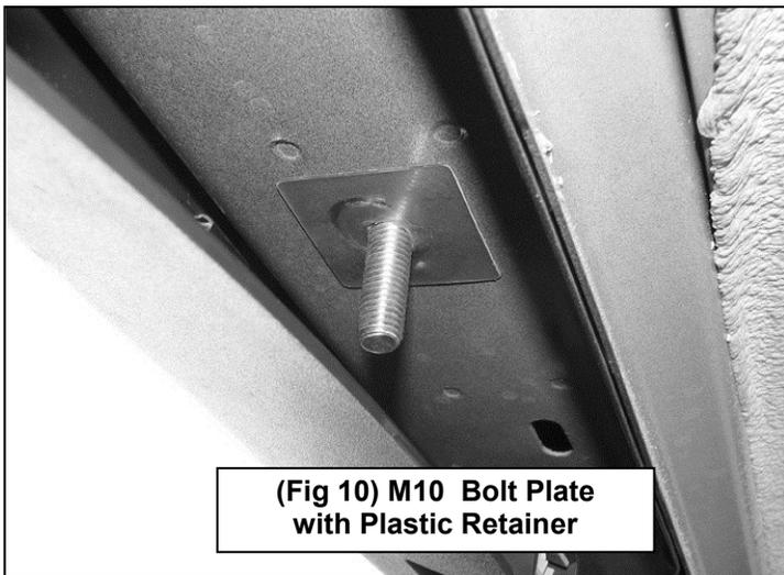
(Fig 10) M10 Bolt Plate with Plastic Retainer
