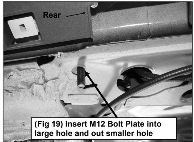
**(Fig 19) Insert M12 Bolt Plate into large hole and out smaller hole**
