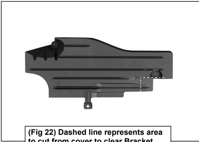
(Fig 22) Dashed line represents area to cut from cover to clear Bracket
