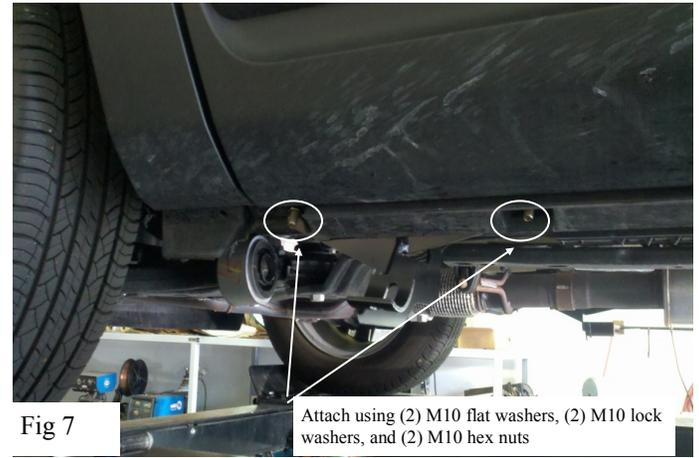
Attach using (2) M10 flat washers, (2) M10 lock washers, and (2) M10 hex nuts
