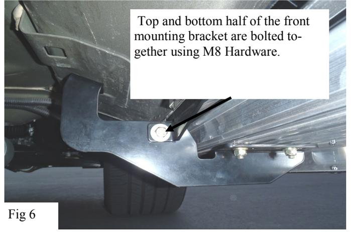
Top and bottom half of the front mounting bracket are bolted together using M8 Hardware.
