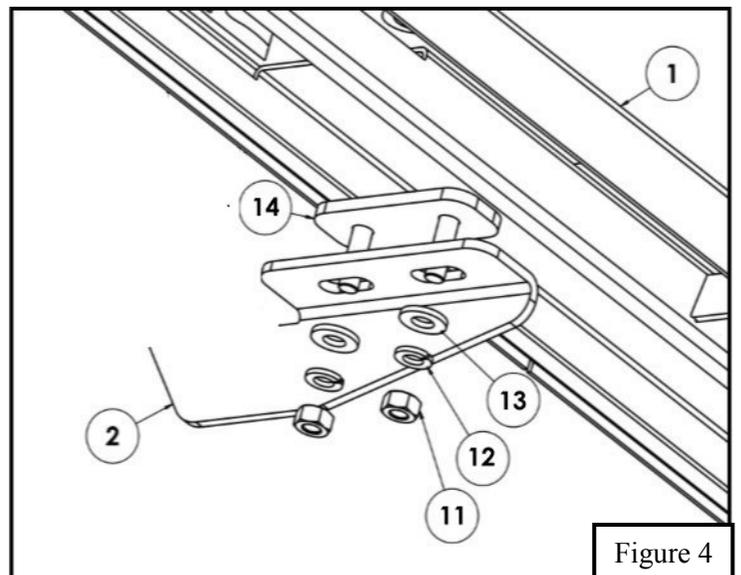
5. Align step bar and brackets to desired positioning then torque and tighten all: M6 hardware to 12 ft-lbs and M8 hardware to 20 ft-lbs.
