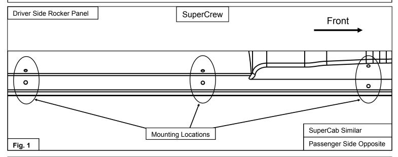
3. Loosely secure (1) Front Mount Bracket (item 1) to the rocker panel using the supplied M10 hardware (items 4-6). See **Figures 1 & 2**.
