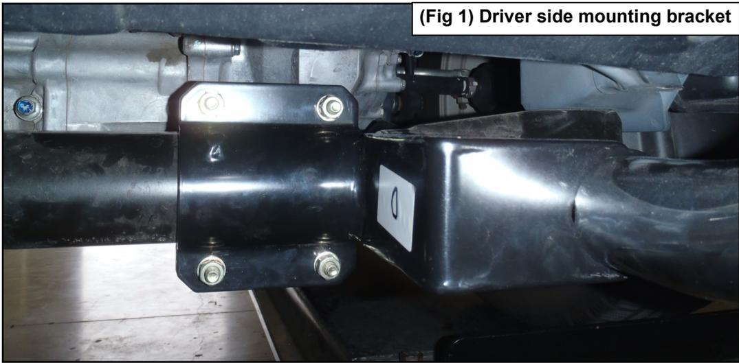
(Fig 1) Driver side mounting bracket
