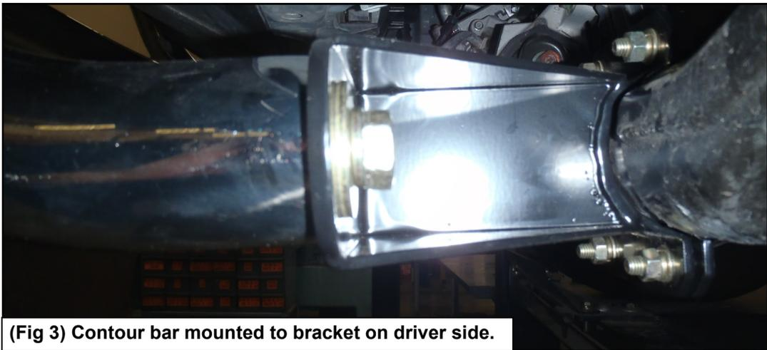
(Fig 3) Contour bar mounted to bracket on driver side.
