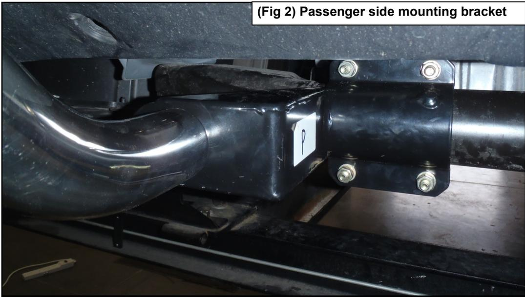
(Fig 2) Passenger side mounting bracket
