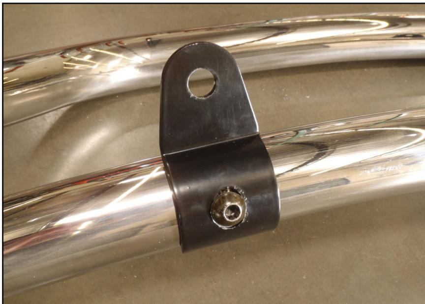
**(Fig 6) Light tab installed on bar**
