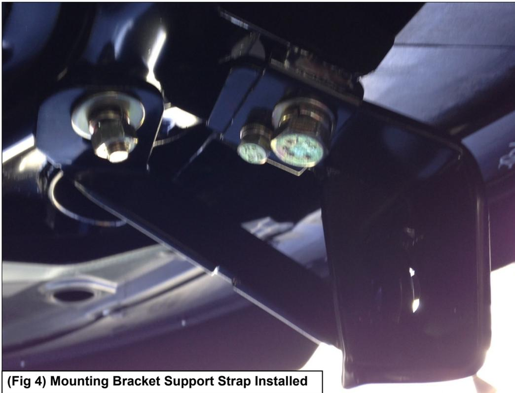
**(Fig 4) Mounting Bracket Support Strap Installed**
