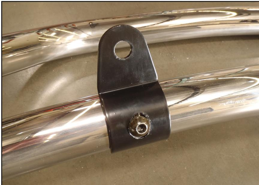
**(Fig 8) Light tab installed on bar**
