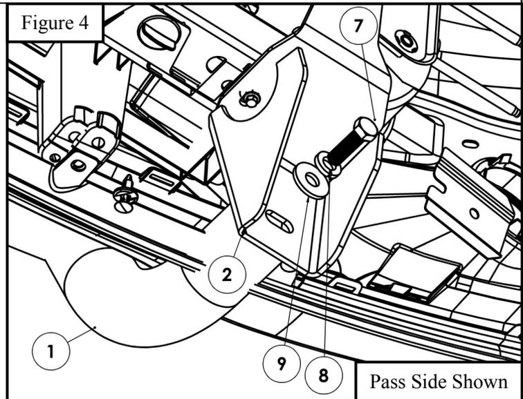
5. Align bar and brackets to desired positioning then torque and tighten all: M6 hardware to 12 ft-lbs, M10 hardware to 30 ft-lbs, and M12 hardware to 65 ft-lbs.
