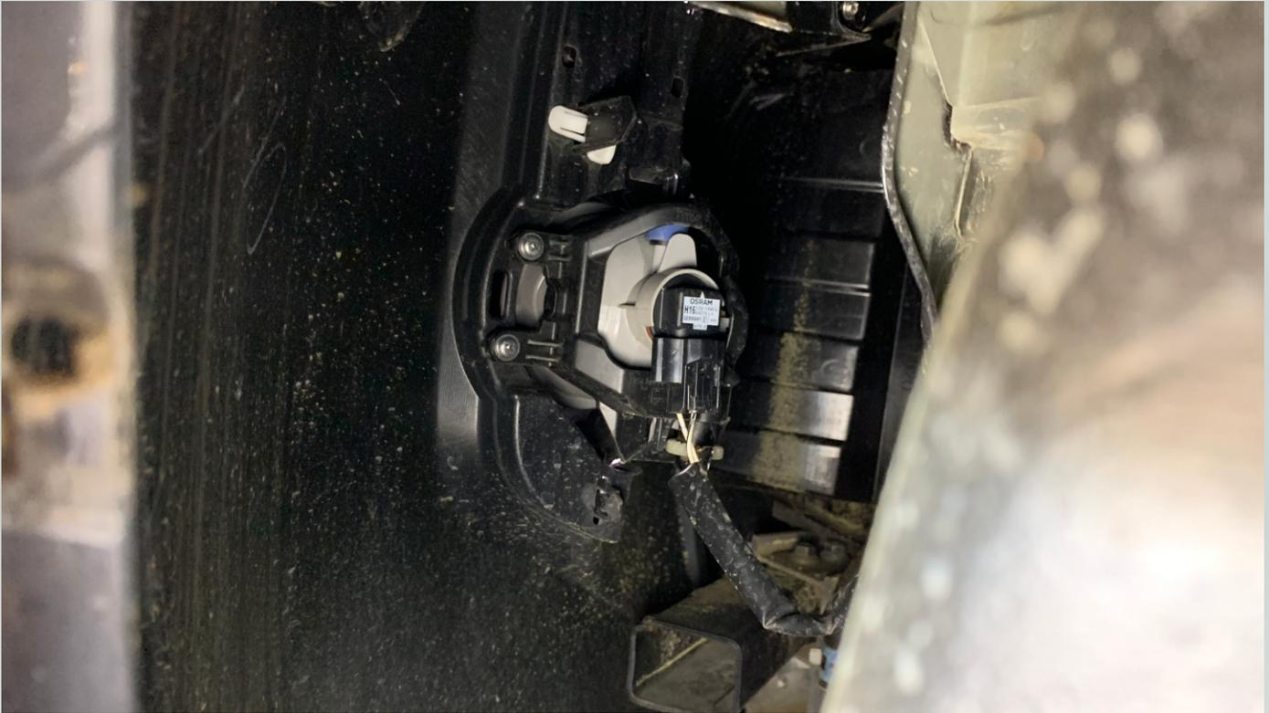
8. Pull the bumper cover over each stud on the sides, then work your way around the bumper cover to remove.
