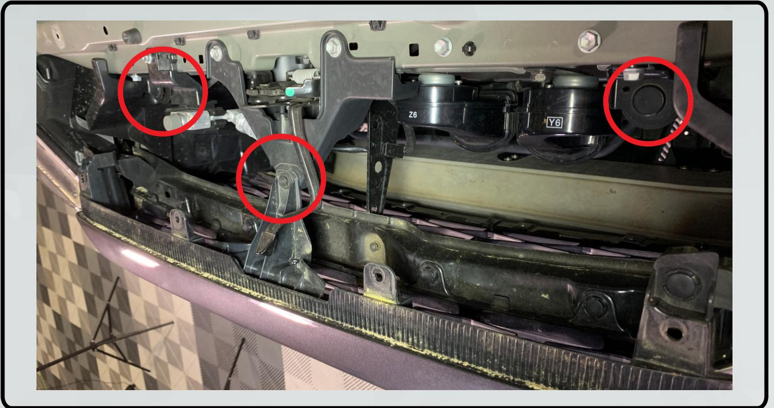
7. Reach in behind fender liner and unplug fog light bulbs. The bumper cover is now ready to remove.
