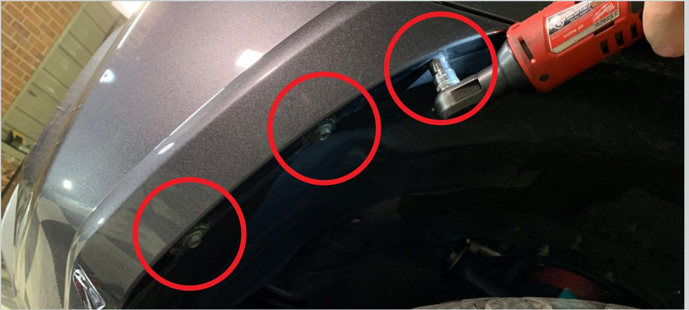
2. Remove the two (2) two-piece push clips from the corner of the top of the grille, one on each side.
