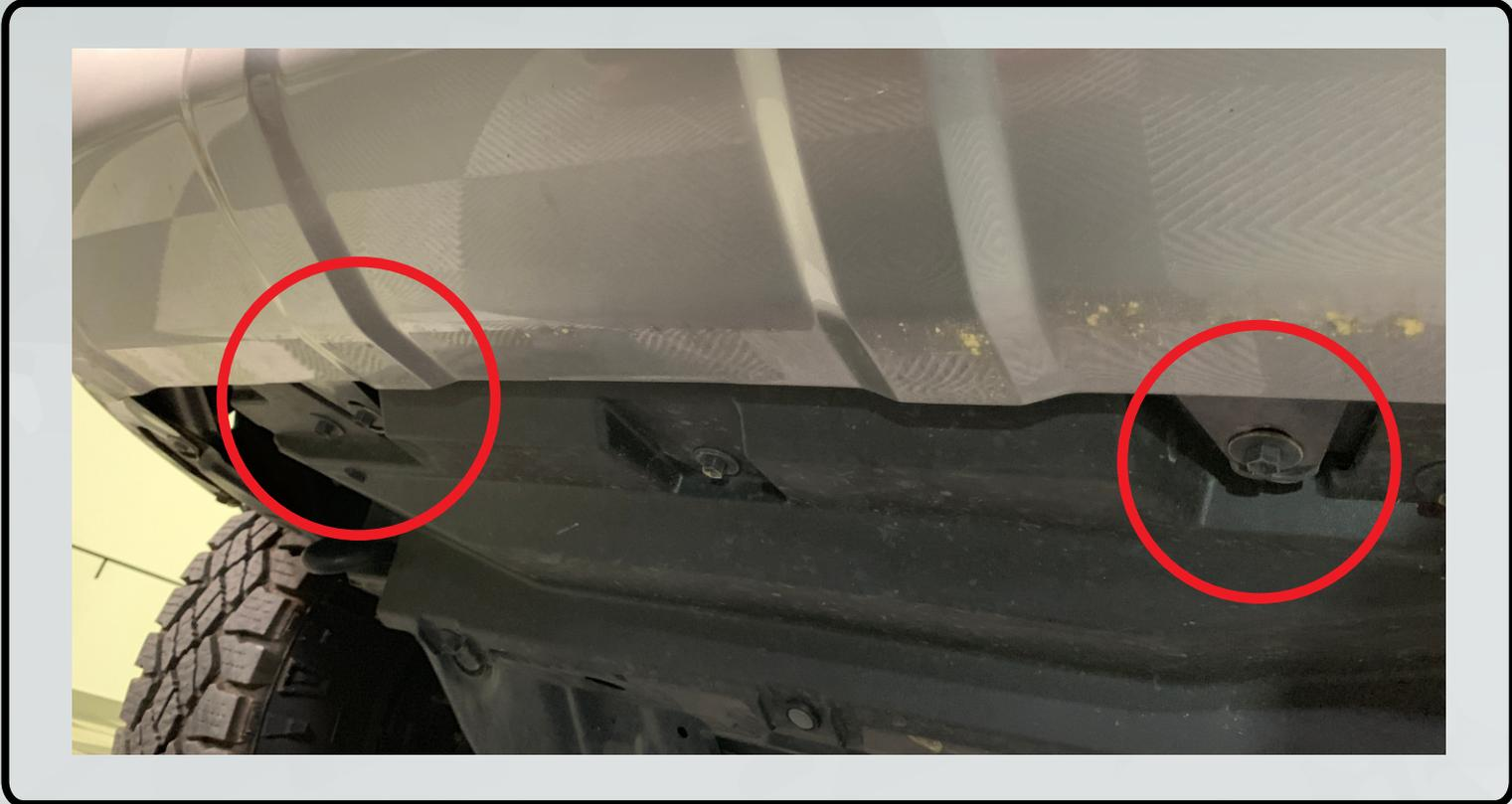
5. Remove the push clips along the top of the radiator shroud. They release by pushing in the center of the clip and then prying the clip out of the hole.
