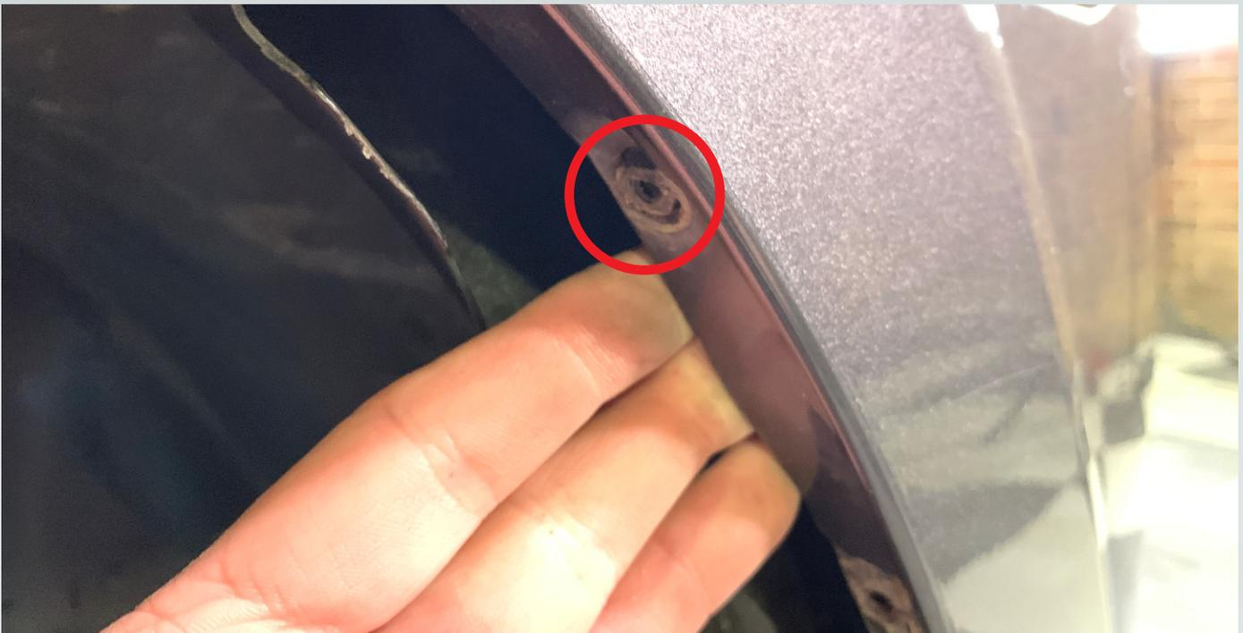
9. Remove the four (4) 10mm screws holding the headlight on the truck. Lift plastic tabs over white screw clips. Unscrew bottom headlight bracket from headlight (2 screws) and fit to Morimoto headlights.
