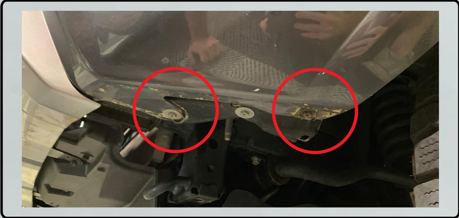
4. Remove the two 10mm screws from under the center of the bumper cover.
