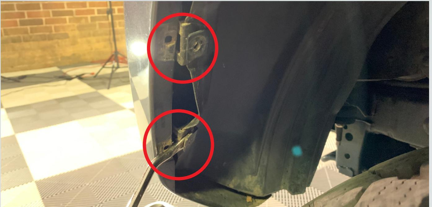
3. Remove the two 10mm screws from under each side of the bumper cover.
