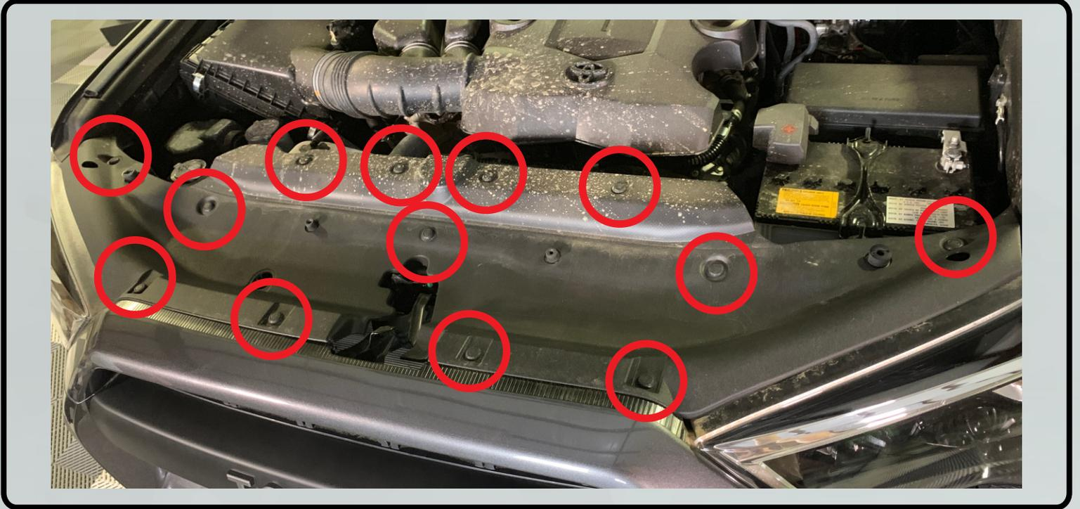
6. Remove the two push clips and 10mm bolt from the grille assembly as indicated.
