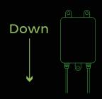
We recommend ensuring the wiring exits the ballast at the bottom to minimize the risk of water ingress.
